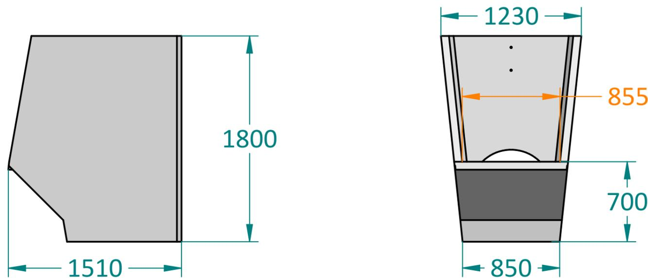
The dimensions in red give the distance from the PE 600-1000 sill level to the INVERT of the pipe.
